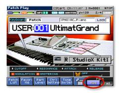
You can select patches on the Patch Play screen by highlighting the patch number—as shown above—or bank name, and then turning the VALUE dial. (We'll explain banks in a few pages).
